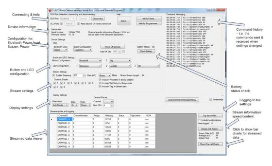
The Handtool can also be controlled directly by a user application using a virtual Com port.
